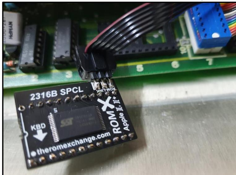
7. Thread the ROM-Link cable underneath the keyboard then carefully line up the pins of the 2316B SPCL module above the socket, and gently press the module down until it is fully seated. A small gap between the underside of the printed circuit board, and the top of the socket is normal.
